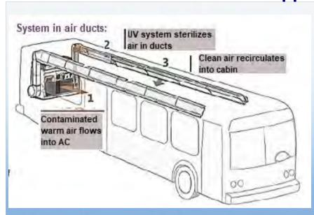
The Breathe-Safe<sup>™</sup> In -Duct discrete System is a patented system that provides new Ultraviolet Germicidal Irradiation Technology (UVGI) for transit vehicles.
